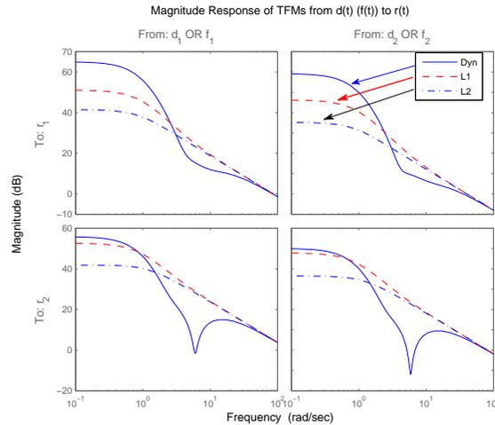
Fig. 4. Magnitude responses of the TFMs  $\tilde{G}_f(s)$  and  $\tilde{G}_d(s)$  in dynamic filter (solid), static filter  $L_1$  (dashed) and  $L_2$  (dash-dot). Note that,  $\tilde{G}_d(s)$  and  $\tilde{G}_f(s)$  are identical, because  $B_d = B_f, D_d = D_f$ .
