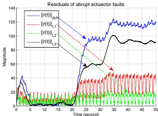
Fig. 6. Residuals of the dynamic filter,  $H_\infty/H_\infty$  filter  $L_1$  and static filter  $L_2$  in the case of two abrupt actuator faults at 20s and 30s, respectively
