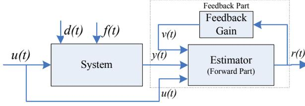
Fig. 1. Structure of the filter problem
