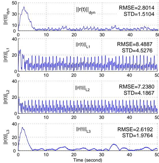
Fig. 5. Fault free residuals corresponding to the dynamic filter , the  $H_\infty/H_\infty$  filter  $L_1$ , static filter  $L_2$  and disturbance estimation approach  $L_3$ , respectively.
