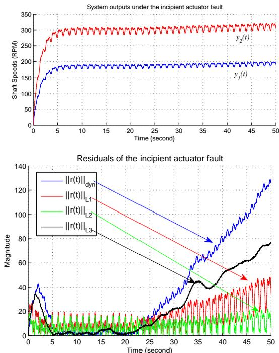
Fig. 7. Plant outputs and residuals under an incipient actuator fault at the first input channel. The actuator fault occurs at 20 second with slope rate 0.005
