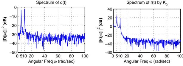
Fig. 3. Spectra of the disturbances and the residuals of  $K_0$ .
